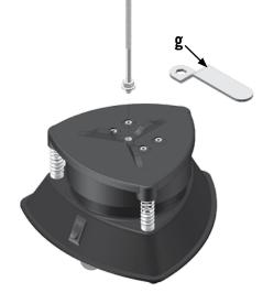
6. The Lid is held in place with the second Washer and Wing Nut.
